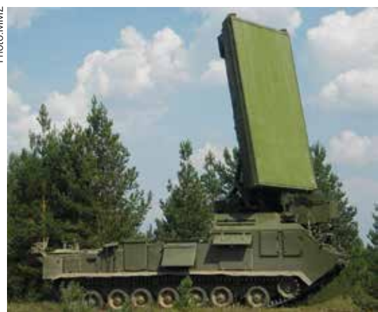
The Russian Army artillery 1L219M Zoopark-1M weapons locating radar is a valuable prize for the Ukrainian military. An example was documented captured by Ukraine in September 2022.
