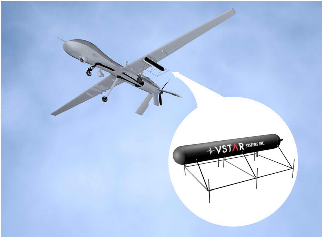
△ HF COMINT systems are outfitting UAVs. This VStar Systems' MA-C MiniPOD being one example. (Image: VStar Systems)
