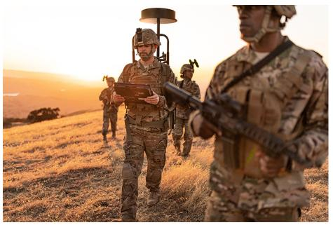
Manpack SIGINT systems provide a highly versatile capability to allow the dismounted collection of signals intelligence to support conventional and special forces.
